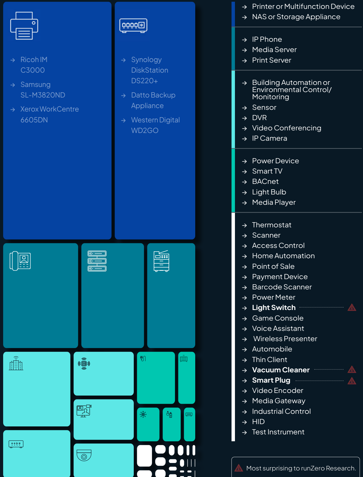
Figure 18: Unusual devices with IP forwarding capabilities. Box sizes indicate relative frequency in our dataset.
